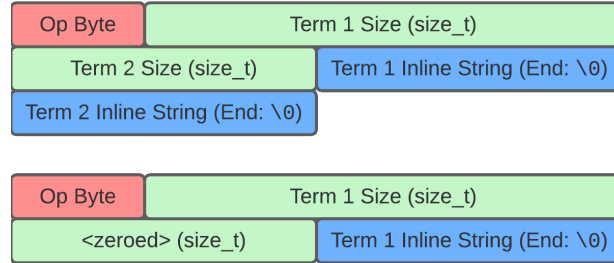
Figure 3.8: Key memory layout. Top structure has both terms present, and bottom structure has only term 1 present.
